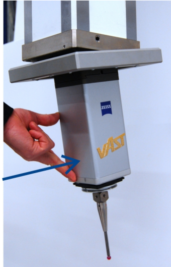
Performance check of the probe protection
