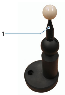
1 Vertical orientation of the reference sphere
