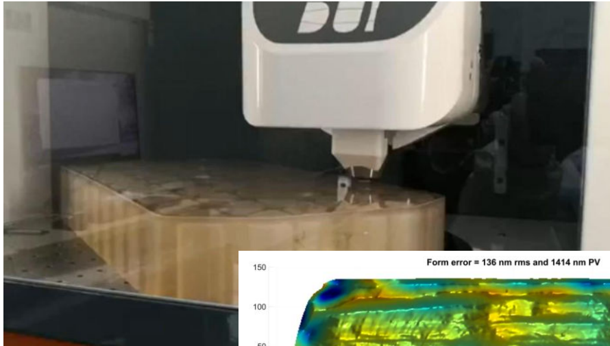
550 x 260 mm aperture, off-axis convex asphere with radius of 75 m (!)
