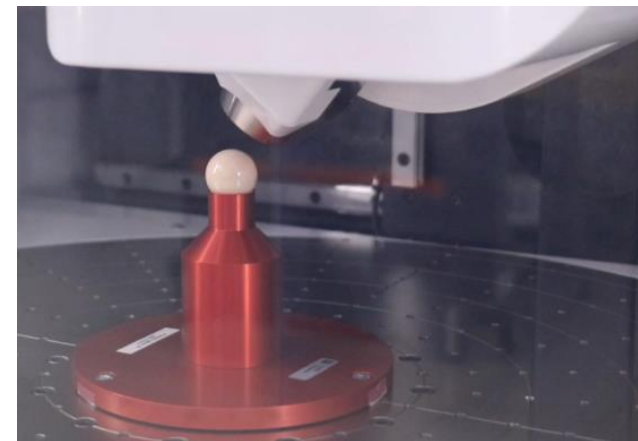
Calibrated 1" radius reference sphere
