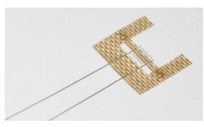
STN series bondable high temperature gages are dedicated for measurements of deformations in the details of machinery and equipment, including jet engines, under static and dynamic loads in -269...+900°C temperature range.
